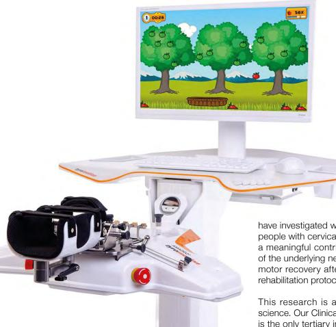
across multiple joints in a functional way may be more beneficial. Tyromotion<sup>®</sup> (Tyromotion<sup>®</sup> GmbH, Graz Austria) have developed a suite of robotic therapy devices capable of training the entire upper limb (shoulder, elbow, wrist, hand and fingers) using separate devices to target each body segment.
